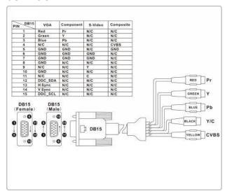
VGA input board of matrix supports the input of analog, composite video and component video; VGA output board supports the output of analog, composite video and component video. If users need input or output component video signal, they need connect DB15 male socket transfer cable (S terminal, RCA head). The two kinds of connection are different, two things should be noticed:
