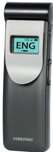
These ergonomically designed pocket receivers incorporate the latest electronics technology. VIS-VLI703A series of IR receivers, which can receive up to 32 language channels and is equipped with channel selector, volume control, power switch, Ø 3.5 mm stereo earphone jack. A LCD displays channel number with language name, received signal intensity, battery capacity and volume. The pocket receivers can be used for both language and music distribution.
