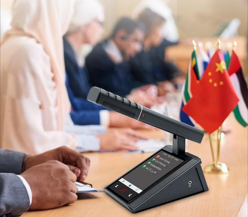
VIS-DMD-T is based on the VISSONIC AUDIOLINK multimedia IP network communication protocol. The unit is equipped with a 5-inch touch screen, which improves the flexibility of conference functions and the content interactivity.
