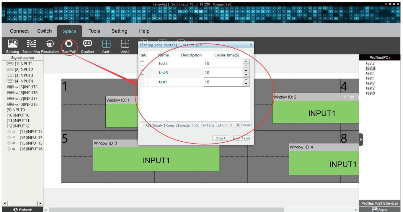
Splicing to set the panel quantity for row and column
