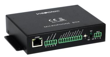
The VIS-AIB microphone interface box is designed to support VISSONIC conference microphone remotely installed under the table or armrest solution. With the phoenix connectors on both sides of the box, it can connect Dynamic mic/Boundary Condenser mic input, buttons and speakers on plate to control the conference unit etc. By the RJ45 port it can easily connect into existing VISSONIC conference microphone family to integrated into one part seamlessly.
