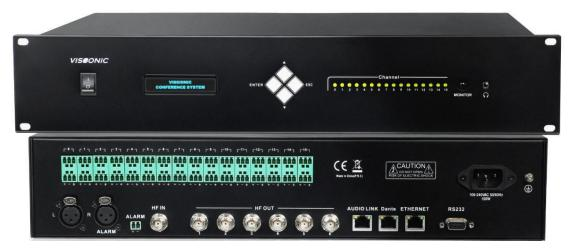
The transmitter is the central device in the language distribution system. It accepts analogue or digital input, modulates these signals onto carrier waves and transmits these carrier waves to radiators located in the room.
