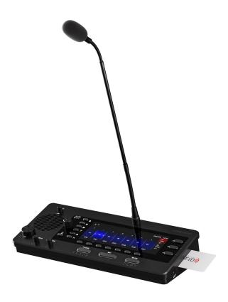
VIS-INT64-P is a translation console with up to 64 channels, transmitting power, audio, and control data via a single Cat5e cable. Its digital design minimizes background noise, distortion, and crosstalk. Featuring a usercentric design and compliant with ISO standards, it includes a 6.8" TFT LCD screen, built-in 64 channel selectors and speakers, and detachable microphone and headphone/microphone jack assemblies, meeting the translation needs of multilingual venues.
