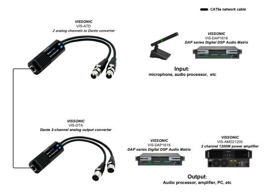
DANTE application network diagram (one-way audio network transmission solution)
