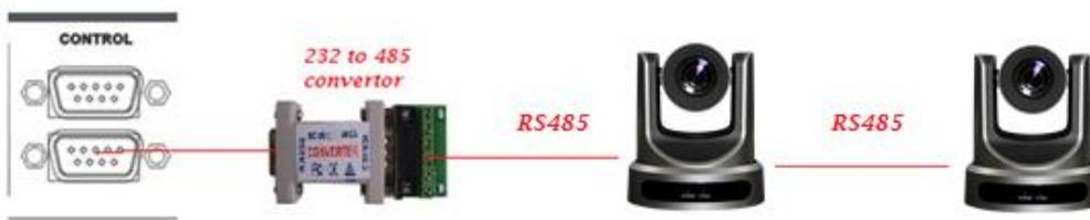
2. Connect the upper COM of CONTROL port of the controller to the camera auto-tracking controller (VIS-CATC-A).
