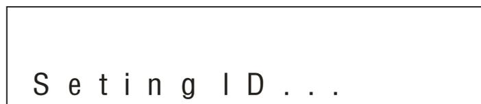
Step 4: Press the MIC key on PMU-T (button turns red) or anywhere on the screen to assign IDs (starting from 1). PMU-T displays its current and new IDs during setup.
